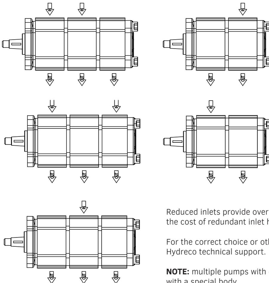
Reduced inlets provide overall systems savings by reducing the cost of redundant inlet hose and fittings.
