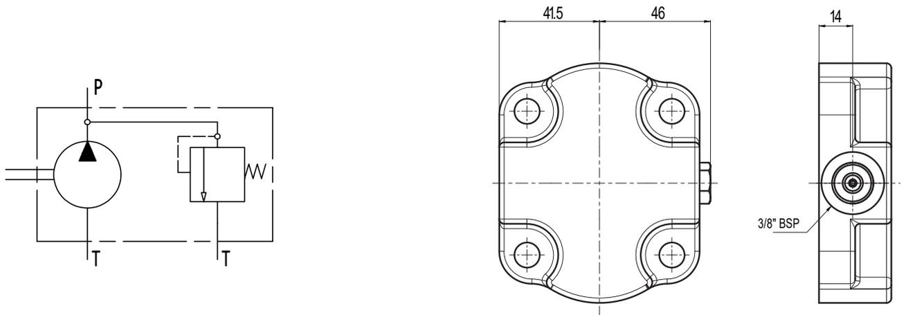
Code **RIF** RELIEF VALVE WITH INTERNAL DRAIN (FIXED SETTING)
