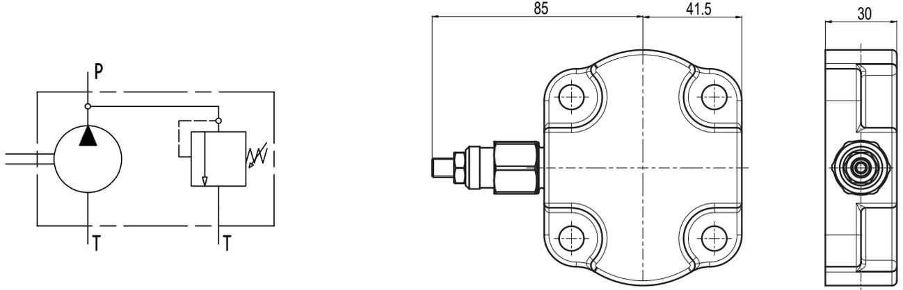
Code **RIV** RELIEF VALVE WITH INTERNAL DRAIN (ADJUSTABLE SETTING)
